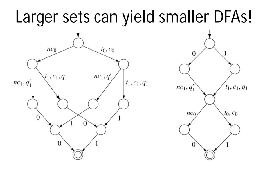
• DFAs after adding the configuration  $\langle c_0, c_1, 1, 1 \rangle$  to the set
