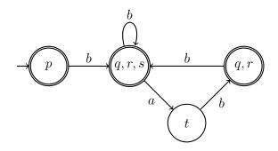
(d) States  $\{p\}$  and  $\{q, r\}$  have the exact same behaviours, so we can merge them. Indeed, both states are final and  $\delta(\{p\}, \sigma) = \delta(\{q, r\}), \sigma)$  for every  $\sigma \in \{a, b\}$ . We obtain:
